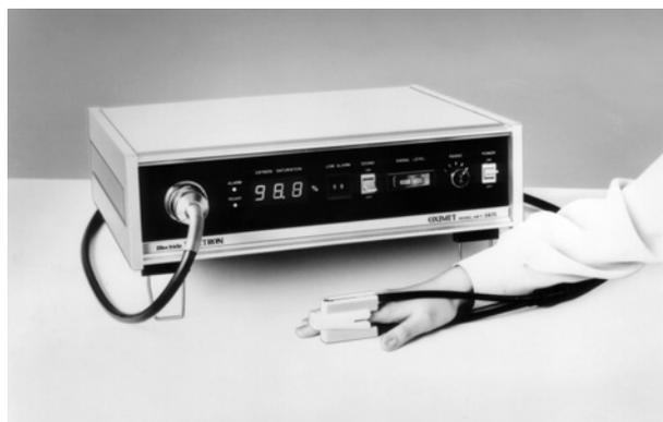
Fig.1 Oximet MET-1471: the world's first fingertip probe pulse oximeter
