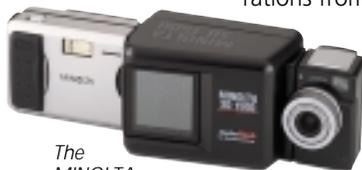
The MINOLTA 3D 1500 is a portable and integrated system that handles the inputting, editing, production, and outputting of 3-D images.
