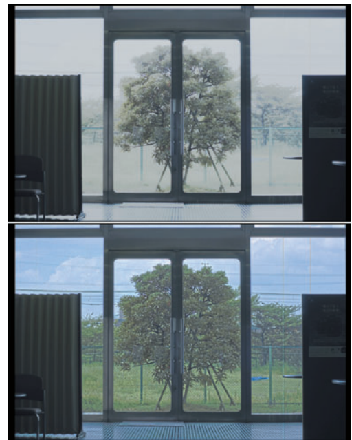
Fig.10 Images from our contrast improvement processing; input image is taken with test sample of linear/log CMOS image sensor. Top: image from conventional image data processing. Bottom: image from our contrast improvement processing
